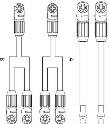
Anderson connector is used on the DC input side of the battery energy storage system.
